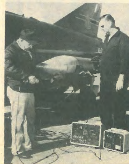
Engineers checking operation of the LGB guidance head using a flight line test kit.
